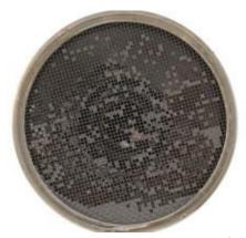
The tiny openings in the oil pickup tube screen can easily plug with sludge, starving the engine of oil.
