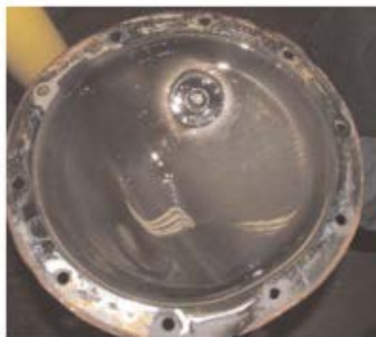
Differential gear lube sumps are equipped with magnets that attract metal wear particles.
