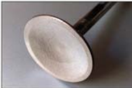
Most engine valves feature valve heads with a concave area that faces into the engine's combustion chamber. If a valve is overheated, this area may become distorted, increasing the depth of the concave area and making its appearance similar to the head of a tulip. This also increases the valve's overall length and reduces valve clearance.
