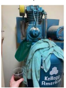
back in service for two weeks, logging a total of 10 hours run time. After that, I proceeded to do an additional three oil changes following the same procedures as before. Finally, after the 7th total oil change the lubricant was at a point that I felt comfortable.
