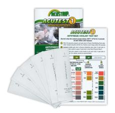
Much like the PH Strips that you may have used in high school science class, after dipping Amsoil Coolant Test Strips in your coolant, the pads will change color. You can then compare the color of the pads to the chart to determine the health of your coolant. For more information, I encourage you to check out the video link (at right).
