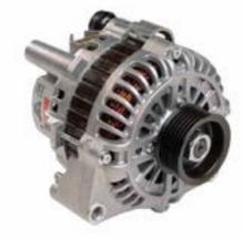
When the car is running, a belt that is connected to the crank-shaft rotates the alternator mechanism. Thus, when the engine is operating, the alternator produces electricity to recharge the battery and to stabilize the voltage in the electrical system. If the alternator fails, the battery can supply power for the car until it becomes discharged.
