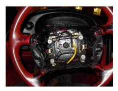
If your steering wheel buttons aren't working properly, you may have a broken clockspring. However...check your fuses first.
