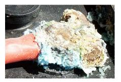
Corrosion and build up on battery terminals can keep your car from starting, or cause you to loose power while driving.
