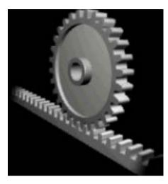
Nearly every new vehicle is equipped with rack-and-pinion steering. Some vehicles use a variation of the rack and pinion and linkage systems. In these vehicles, a rack-and-pinion is used to provide the directional force. A simplified linkage system transfers the force to steer the wheels.
