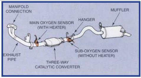
through the second Oxygen Sensor and on to the Muffler. The Muffler has the job of reducing engine noise without restricting exhaust flow enough to cause excessive back pressure.
