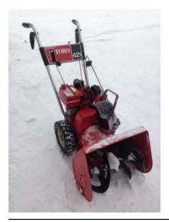
Last summer, I worked on the Toro for about an hour before getting it working. I drained the gasoline and replaced with new. I cleaned the carburetor bowl as well as the carburetor itself. I ensured there was good fuel flow to the carburetor. I changed the oil (given that it is a 4-cycle engine). Checked all the mechanical linkages for proper operation. Lubricated the moving parts and of course cleaned the spark plug and checked the gap.
