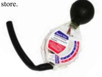
If you are running Amsoil's Low Toxicity Antifreeze and Engine Coolant you will need to test it using Amsoil's Antifreeze Test Strips, as the Low Toxicity Antifreeze and Engine Coolant is a Propylene Glycol formulation rather than an Ethylene Glycol formulations.
