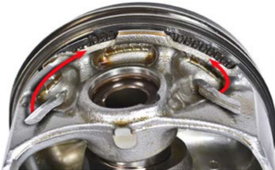
Example of piston damage due to an LSPI event observed during dyno testing. The red arrows indicate sections of the ring land that have broken away from the piston.
