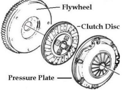
The ring gear for the starter motor is an integral part of the flywheel assembly and the flywheel housing is mounted to the cylinder block. It supports the starter motor and protects the clutch or torque converter.
